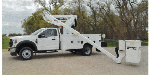
Negative boom angle allows for ground level access from the basket.
